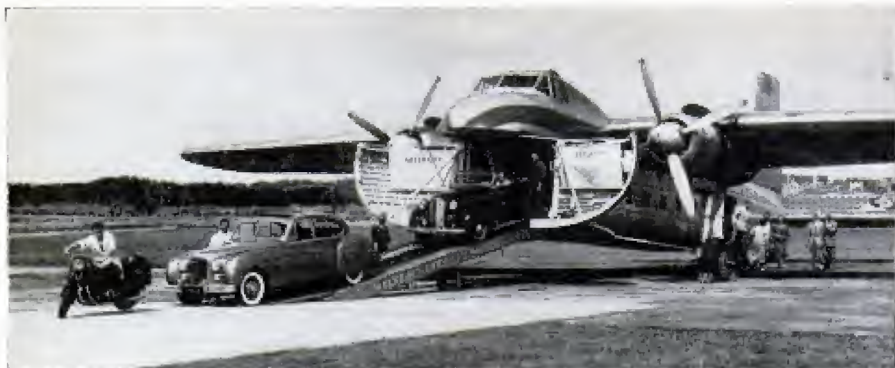
Plane carries two large or three small cars. Air lift is popular with tourists who take their cars with them
